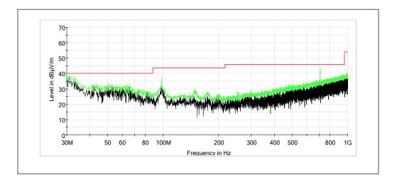
Characterization Scan: 120V/60 Hz, 30 MHz to 1000 MHz, Horizontal
