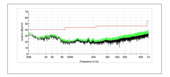
Characterization Scan: 230V/60 Hz, 30 MHz to 1000 MHz, Horizontal
